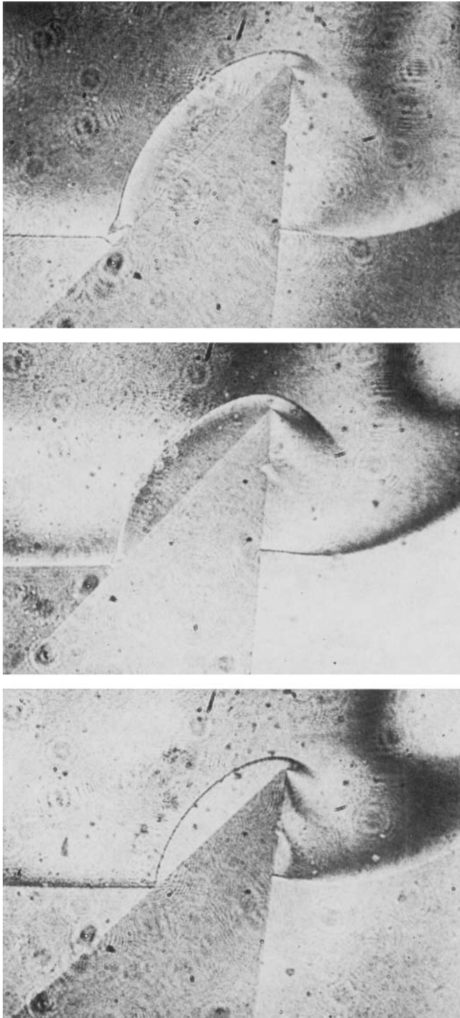
FIGURE 8. Interferograms of shock reflexion in pseudosteady flow of argon. M_2 = 6.7 , p_1 = 10 torr. (a) \alpha = 42^\circ , regular reflexion (incipient Mach reflexion). (b) \alpha = 44^\circ , double Mach reflexion. (c) \alpha = 46^\circ , double Mach reflexion.
